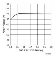
Figure 5. Gate Drive Voltage vs Bias Supply Voltage
