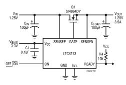
Figure 1. The LTC4213 in an Electronic Circuit Breaker Application
