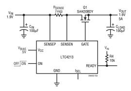
Figure 3. Accurate ECB with High Side Sense Resistor
